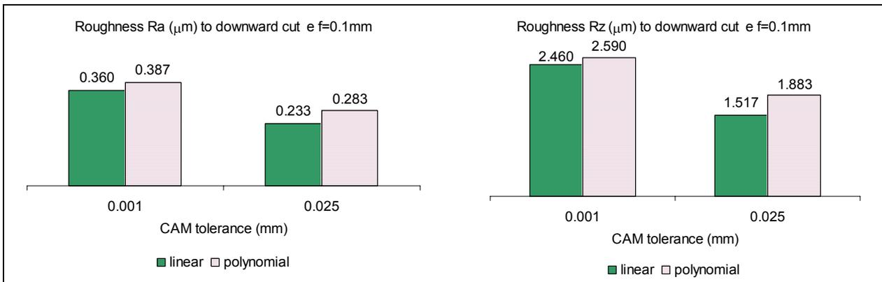
Figure 9.  $R_a$  and  $R_z$  roughness for downward cut.
