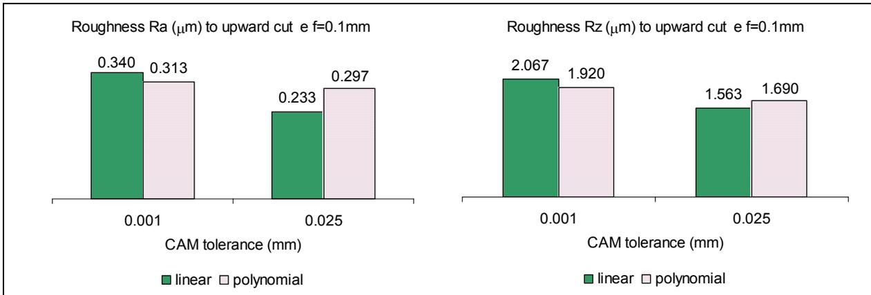
Figure 8.  $R_a$  and  $R_z$  roughness for upward cut.
