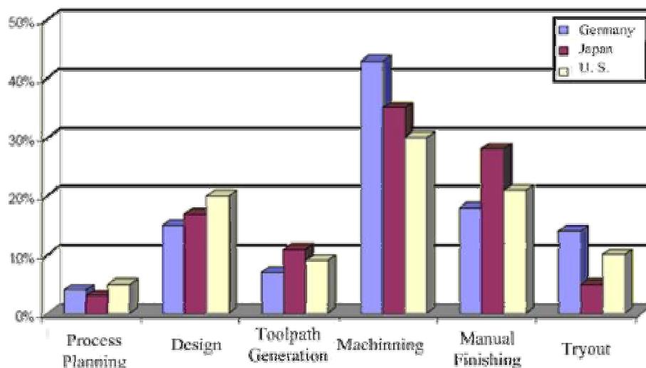
Figure 1. Typical lead-time in the die and mould manufacturing (Fallböhmer *et. al*, 2000).
