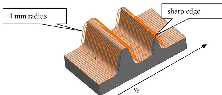
Figure 3. Test-piece geometry and feed direction.
