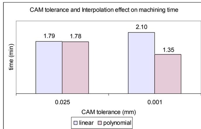
Figure 6. Influence of CAM tolerance and interpolation method on machining time
