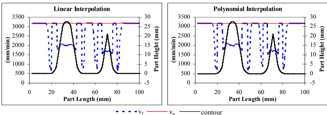
Figure 4. Feed speed behavior along test-piece contour for a 0.025mm CAM tolerance.
