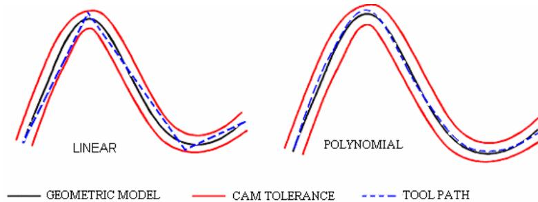
Figure 2. Linear and polynomial interpolation methods.
