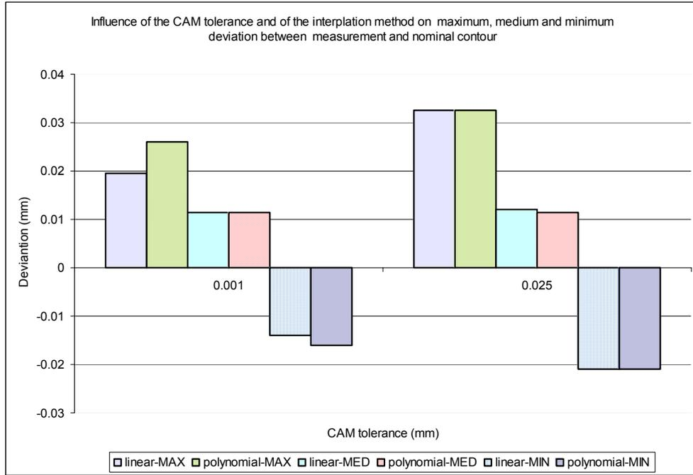
Figure 7. Influence of the CAM tolerance and of the interpolation method on maximum, medium and minimum deviation between measured and nominal contour
