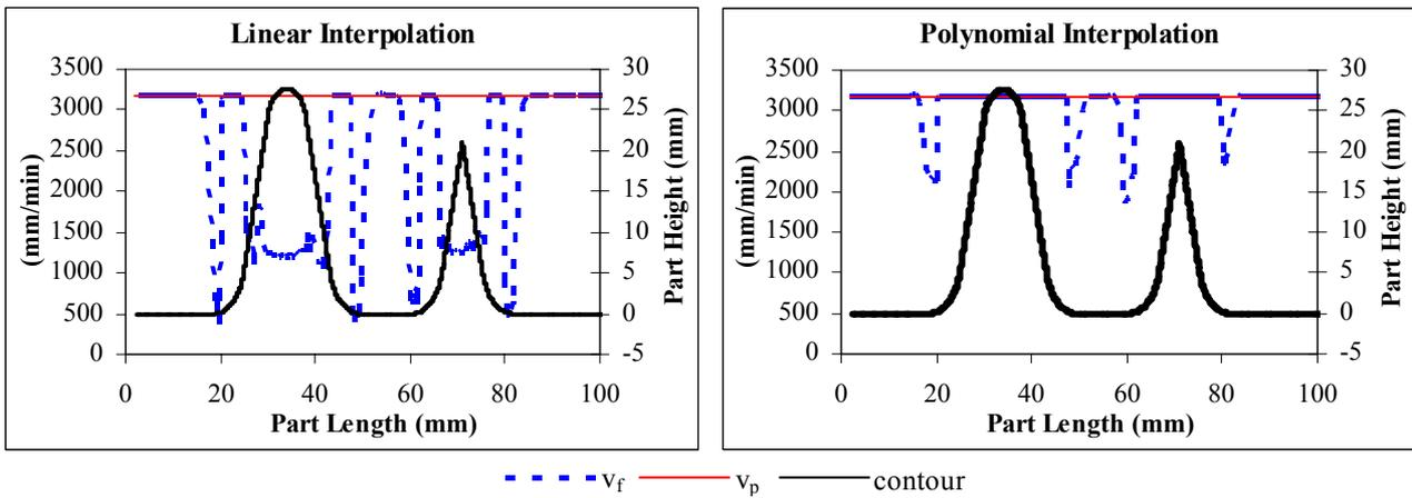
Figure 5. Feed speed behavior along test-piece contour for a 0.001mm CAM tolerance.
