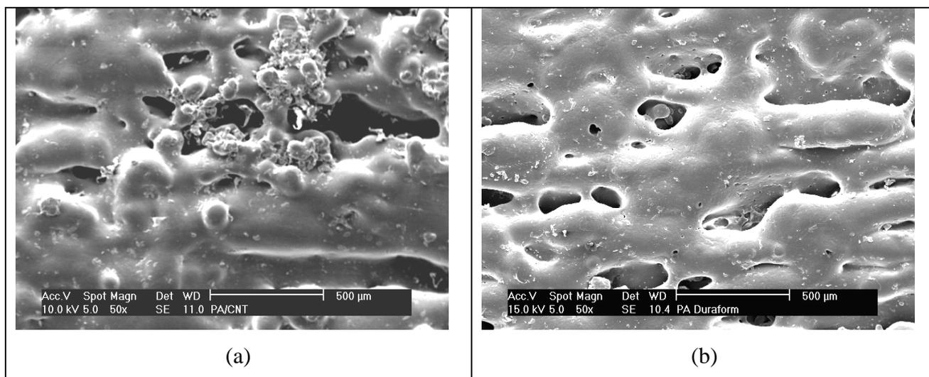
Figure 6 – Surface of PA/0.5%CNT composite (a) and pure polyamide (b).
