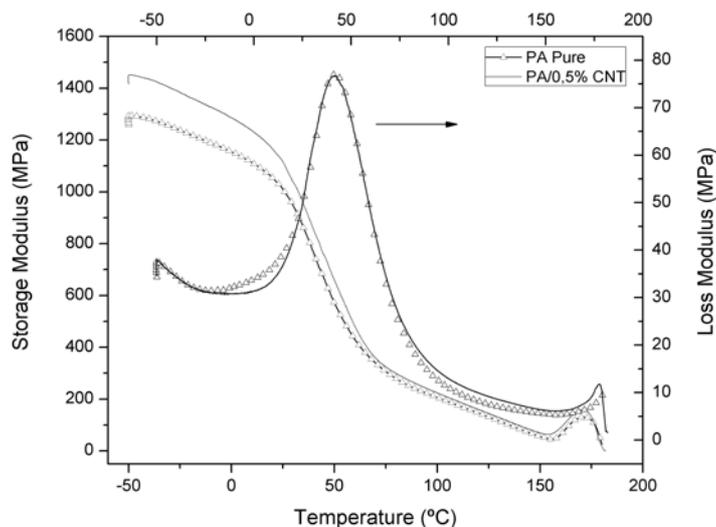
**Figure 8** – Storage ( $E'$ ) and loss ( $E''$ ) modulus as function of temperature for PA and PA/0.5%CNT composite.
