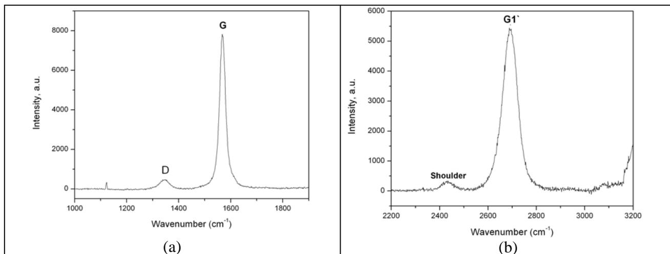
**Figure 2** – First order (a) and second order (b) Raman spectra of the as-received MWNTs.
