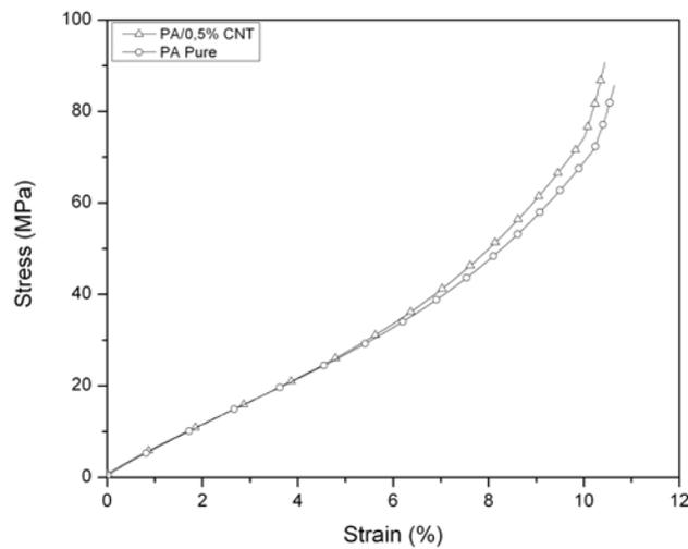
**Figure 7** – Stress – strain comparative curve for PA and PA/0.5%CNT composite.
