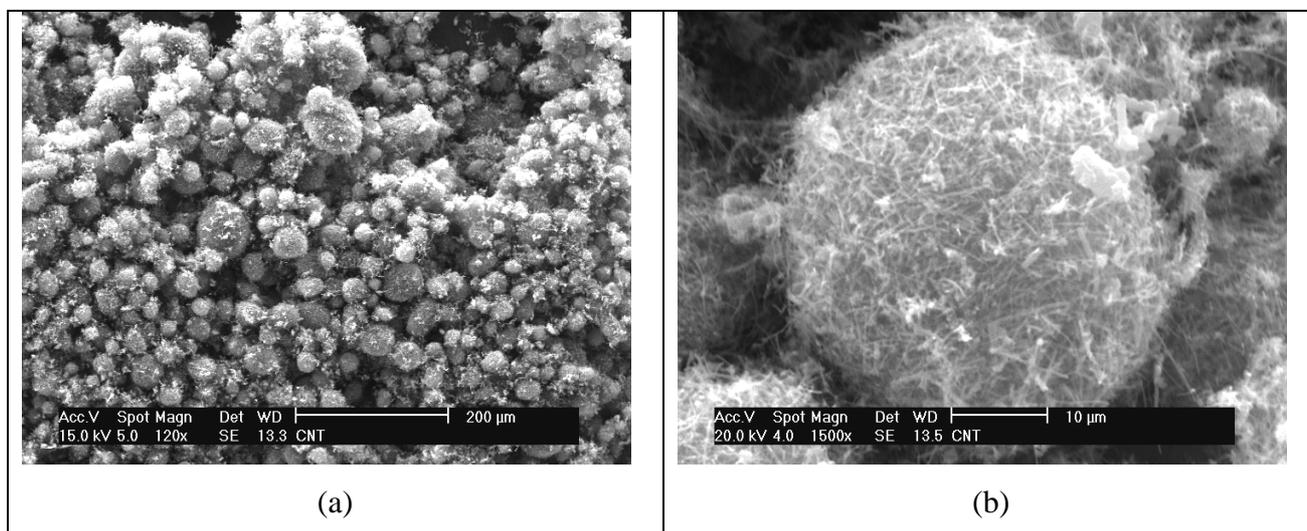
Figure 1 – SEM image of (a) as-received MWNTs, (b) Bundled MWNTs.
