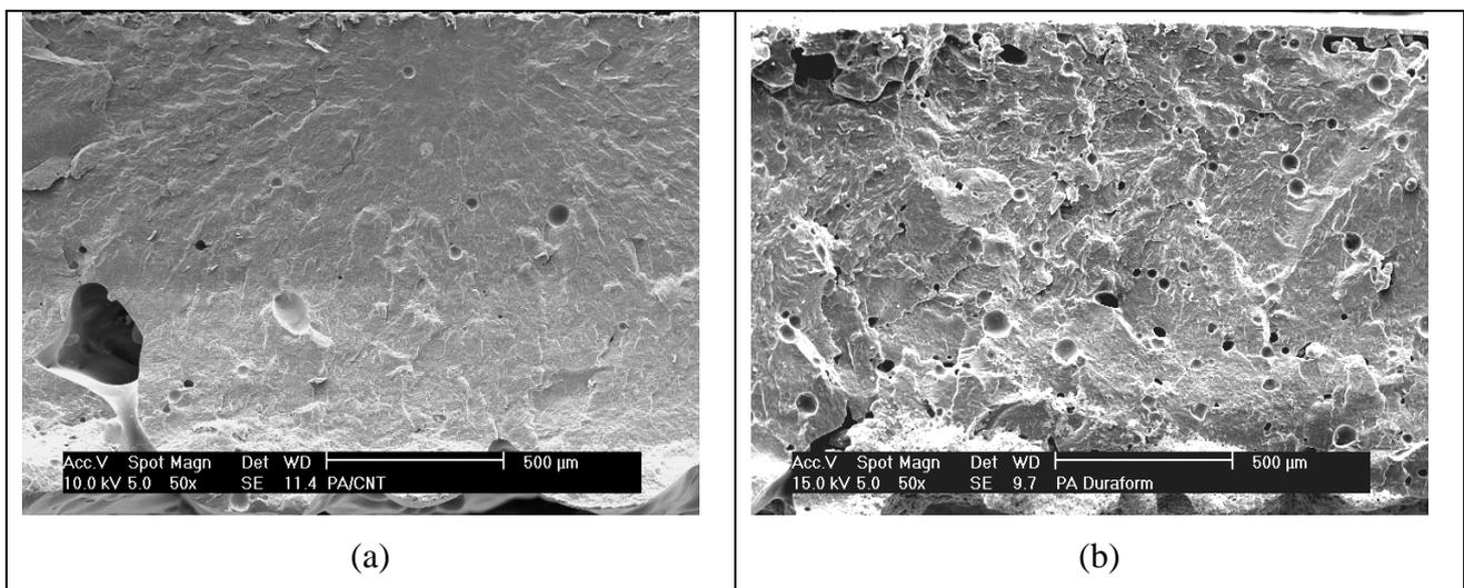
Figure 4 – Cryogenic fracture surface of PA/0.5%CNT (a), and PA (b).
