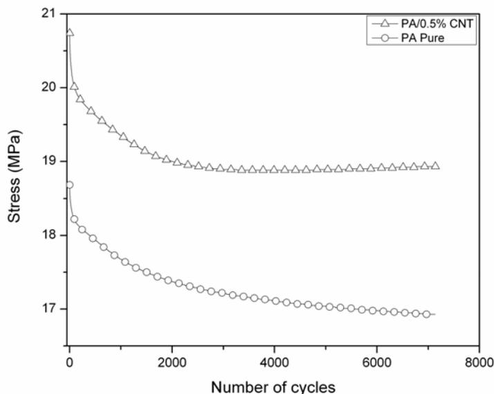
**Figure 9** – Fatigue behavior PA and PA/0.5%CNT composite.
