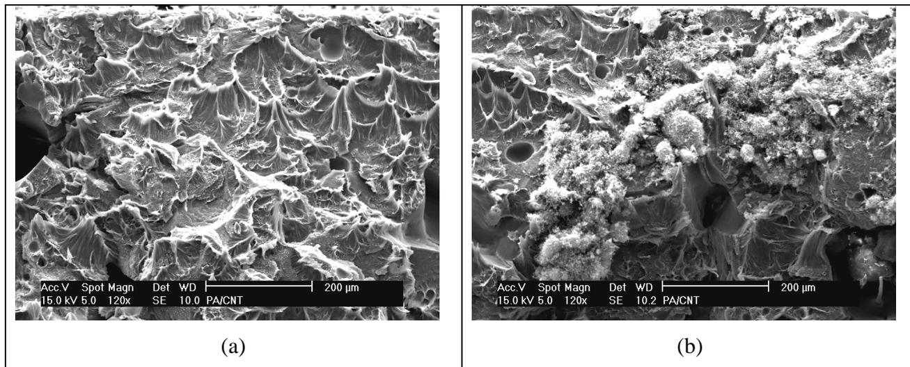
Figure 5 – Mechanical fracture surface of PA/0.5%CNT (a), agglomerate at surface (b).
